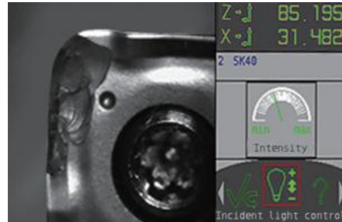
check cutting edge wear
